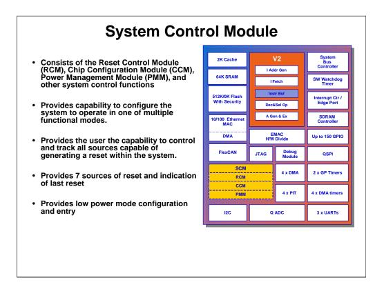
The System Control Module (SCM) is composed of three main blocks: the Reset Control Module (RCM), Chip Configuration Module (CCM), and Power Management Module (PMM).
