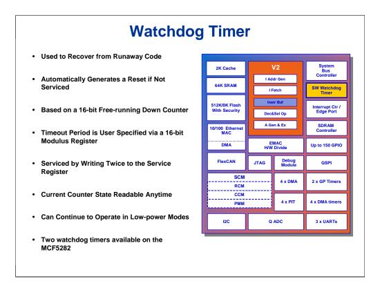
Now let's look at the ColdFire's watchdog timer. The watchdog timer is a 16-bit timer used to help software recover from runaway code. The watchdog timer has a free-running downcounter (watchdog counter) that generates a reset on underflow. To prevent a reset, software must periodically restart the countdown by servicing the watchdog.
