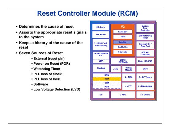
Now we'll examine the Reset Controller Module (RCM). The RCM is provided to determine the cause of reset, assert the appropriate reset signals to the system, and then to keep a history of what caused the reset. The Power Management Module (PMM) control registers are implemented in the RCM. These registers mainly control the operation of the Low Voltage Detect (LVD) circuit.
