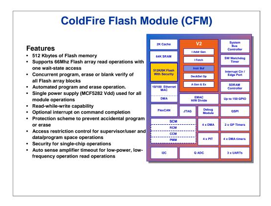
Let's now turn our attention to the ColdFire Flash Module (CFM). This module is ideal for program and data storage for single-chip applications and allows for field reprogramming with no external high-voltage sources. The voltage required to program the CFM is generated internally by on-chip charge pumps.
