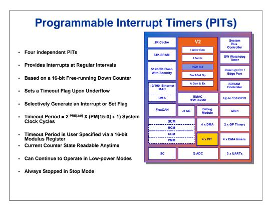
Another module in the MCF5282 is the programmable interrupt timer (PIT). There are four programmable interrupt timers each of which generate interrupts at precise, regular intervals.
