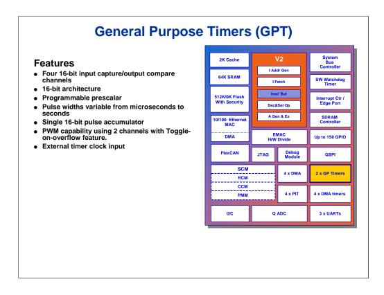
Finally, we'll look at the General Purpose Timers (GPT) of ColdFire. The MCF5282 has two 4-channel general purpose timer modules. Each consists of a 16-bit programmable counter driven by a seven-stage programmable prescalar. Each of the four timer channels can be configured to perform input capture or output compare. Additionally, one of the channels, channel three, can be configured as a pulse accumulator.
