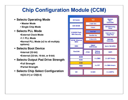
The Chip Configuration Module (CCM) controls chip configuration and low power mode operation.
