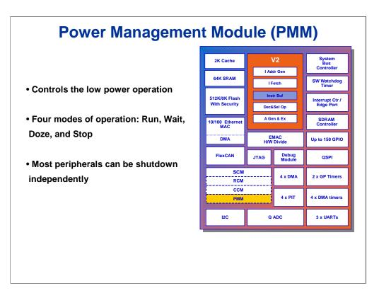
The Power Management Module (PMM) controls the low power operation on the MCF5282.
