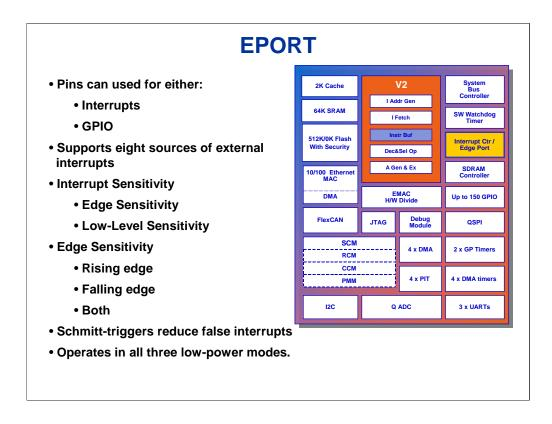
The Edge Port (EPORT) on the MCF5282 is a collection of seven pins that can be used as interrupt pins or GPIO pins.
