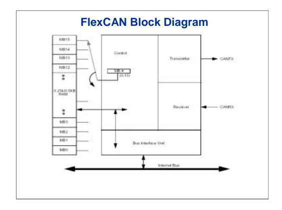
The module operation relating to message reception and transmission is identical to the TouCAN module. FlexCAN offers an increased number of RAM based message buffers (up to 16), all of which can be configured as either transmit or receive. This module can generate up to 19 interrupt sources (16 interrupts due to message buffers and three interrupts due to Bus-off, Error, and Wake-up).
