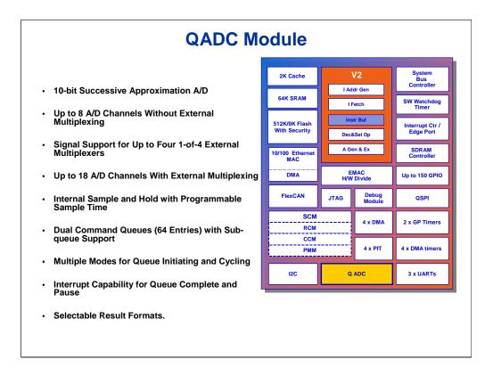
The Queued Analog to Digital Converter Module (QADC) in the MCF5282 is a 10-bit, unipolar successive approximation A/D converter. The interface to the module consists of eight multi-function input/output pins, two reference voltage pins, and two power pins. There is built-in multiplexing and channel decode logic which can be enabled and used to reduce the number of analog inputs to the device. When multiplexing is deselected, up to eight channels can be individually fed in and read.
