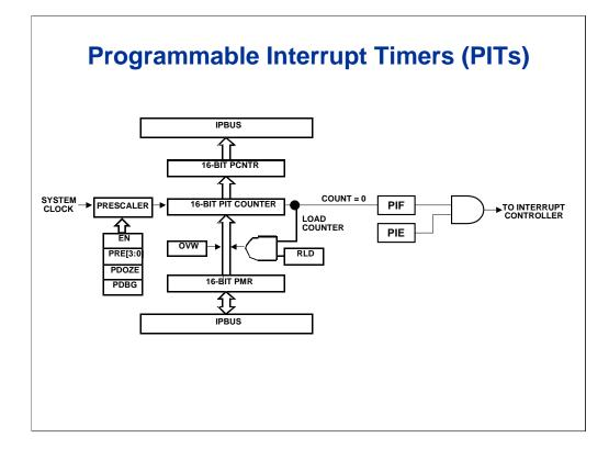
The programmable interrupt timer (PIT) is a 16-bit timer that provides precise interrupts at regular intervals with minimal processor intervention. The timer can either count down from the value written in the modulus register, or it can be a free-running down-counter. This device has four programmable interrupt timers, PIT1-PIT4.
